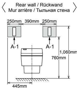
**19** Temporarily place the remote control in the position determined in **18** and confirm the signal reception of A-1.
