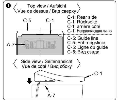
Insert C-1 into A-7 until a click sound is heard. (After C-1 is mounted, make sure that it can not be removed even if it is pulled.)
